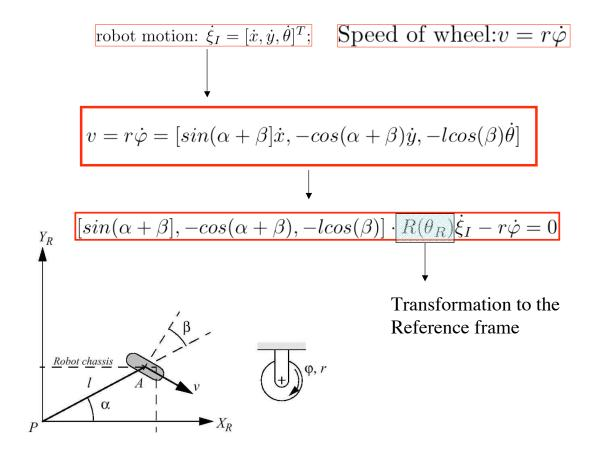
Motion caused by wheel motion, rolling constraints:
