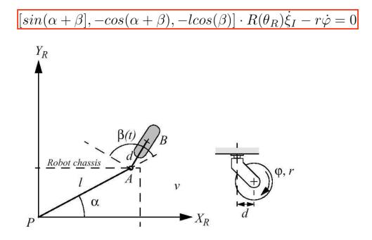
... But the sliding constraint(is different):
