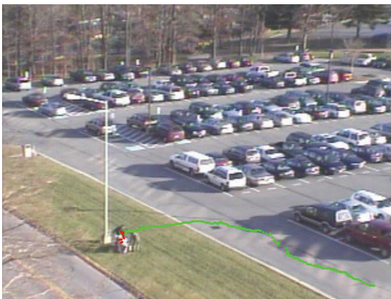
FIGURE 9: The first abnormal test scenario. A person stops moving at a point on his route. We see the increase in the normalized mean square error (NMSE) values when he/she stops, resulting in a deviation from the normal trajectory.
