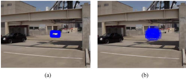
Fig. 4. Comparison of the proposed particles when the adaptive velocity model is used. Note that the particles are tightly clustered around the target when we use the adaptive velocity model. In contrast, without velocity prediction, we need to use more particles to represent the same posterior, because most particles have very low weights. (a) With the adaptive velocity model. (b) Without the adaptive velocity model.
