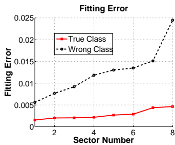
Fig. 15. Plot of the fitting error for the true class and the wrong classes. Note that the true class gives a much lower fitting error on the test iris images. Also, the number of images in the true class is far fewer than the total number of images in the gallery. So the sparsest solution, which gives the least fitting error corresponds to non zero coefficients only for the true class, in most cases.
