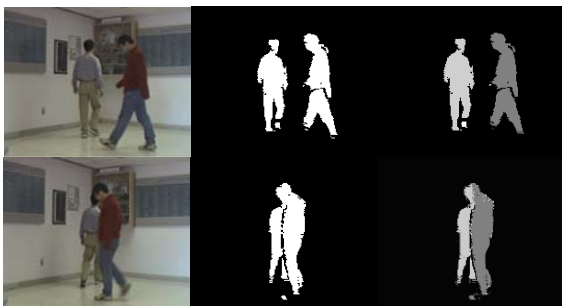
Fig 4. Multiple human detection from indoor sequences. Left column: two input frames (#16 and #25) taken by the left image; Central column: foreground subtraction; Right column: human detection.
