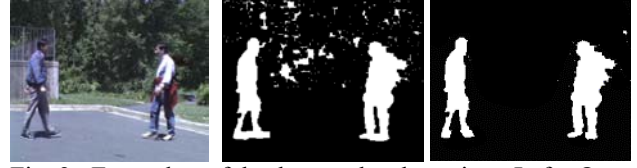
Fig 2. Examples of background subtraction. Left: One input frame; Center: Result obtained using traditional approach; Right: Foreground extraction using the proposed approach.
