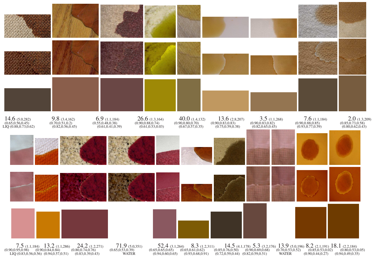
Figure 6. Web images, top to bottom rows: input, synthetic wetting, and liquid albedo.
